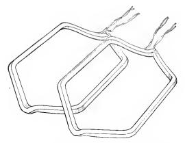
FIG. 145. Armature coils of series railway motor.
